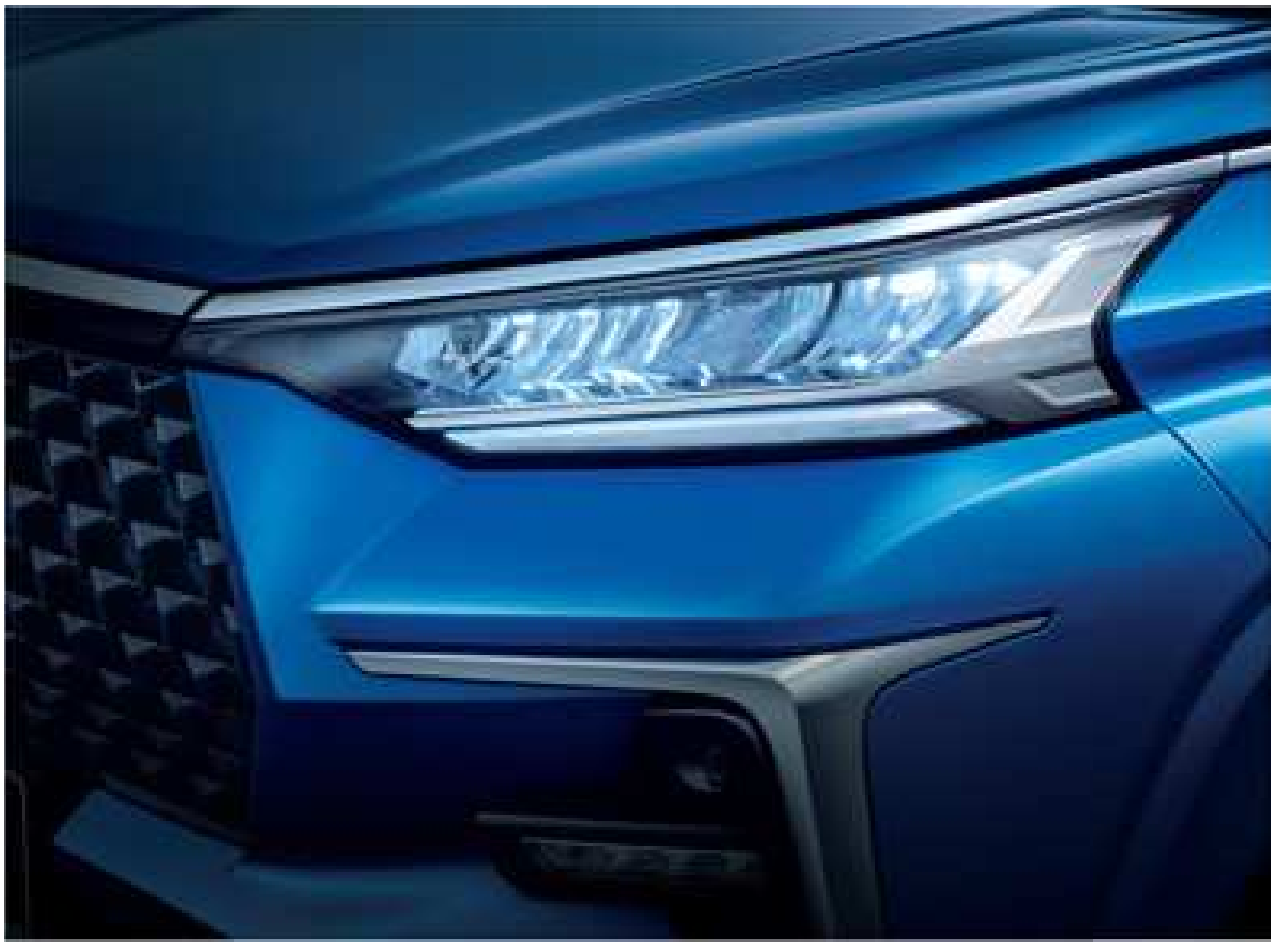
Full LED Headlamps With Sequential Turn Signals and Daytime Running Lights.
