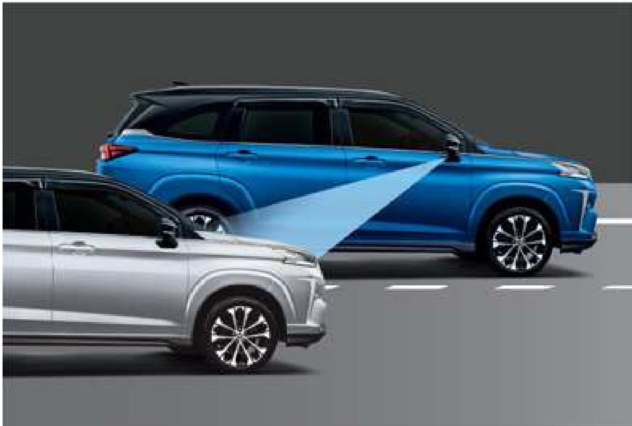
Blind Spot Monitor (BSM) Detects vehicles that may not be visible to the driver when changing lanes or reversing.
