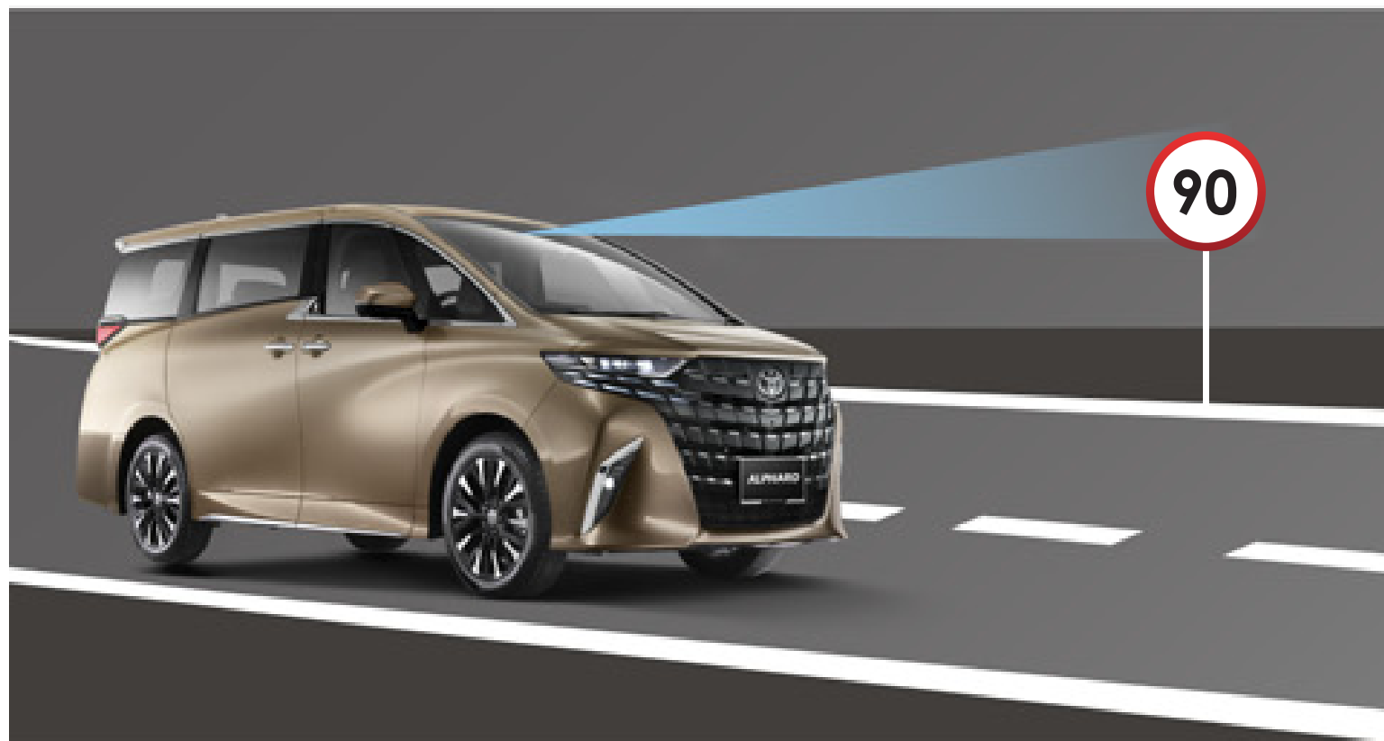
ROAD SIGN ASSIST (RSA) Monitors the road ahead, displaying information such as current speed limit and suggesting necessary adjustments.
